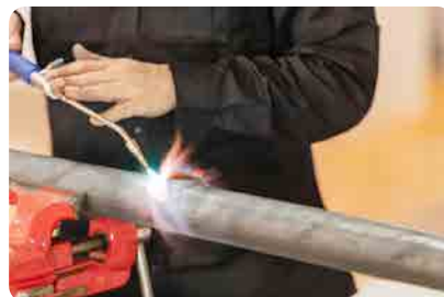
Figure (12) Oxyacetylene flame is used in cutting metals
